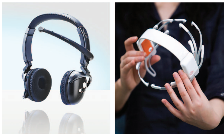
Figure 2. Brain-computer-interface headsets: (a) the MindSet and (b) the Epoc. These devices let players translate their intentions into game actions directly, bypassing traditional input devices such as a mouse, joystick, or keyboard. (Sources: NeuroSky [2a] and Emotive Systems [2b]; used with permission.)
